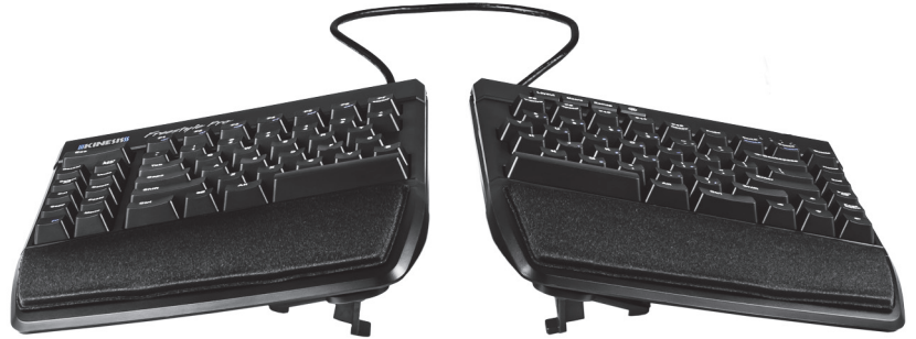
VIP3 Pro kit installed on Freestyle Pro keyboard, 10 degree tenting shown.
