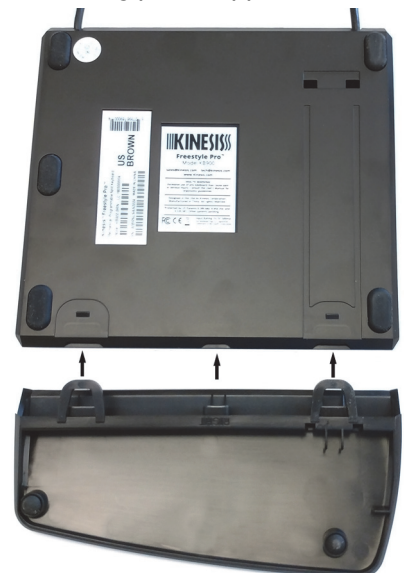
Installing palm supports
