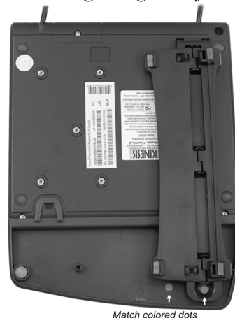
Installing 3-angle V-lifters
